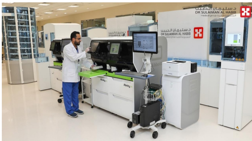
Figure 2. The full automated laboratory instruments connected to the spiral sample track system.
